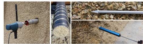
Fig 2. Core sampler (4L volume) and penetrometer to estimate silage density
